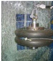
Impact tests (1B1 according to EN 12600)
