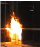
Fire test (B s1 d0 according to EN 13501)
