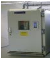
Thermal cycles (from - 40°C to +85°C), humid environment (1000 hours at 85°C and 85% RH)
